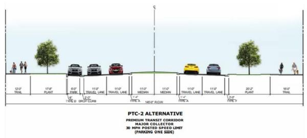
The developers are proposing an alternative roadway design for the premium transit corridor that eliminates bike lanes in favor of a wider landscaped buffer and multi-use trails on both sides of the street. This version includes on-street parking on one side. (Heidt Design)
